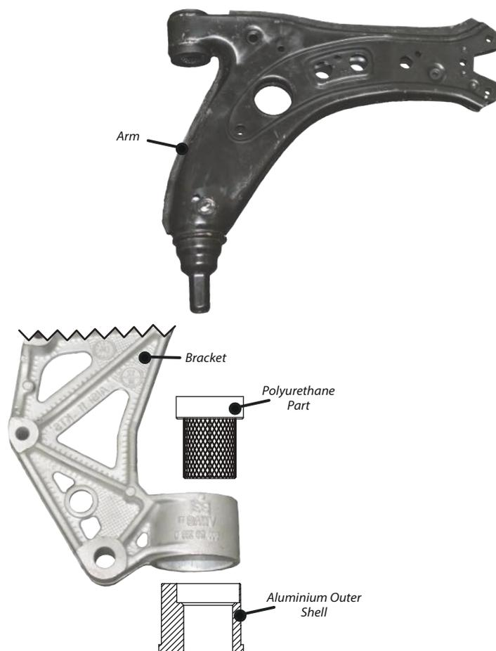
Figure 1 - diagram showing how the polyurethane part and the metal outer shell will fit together
