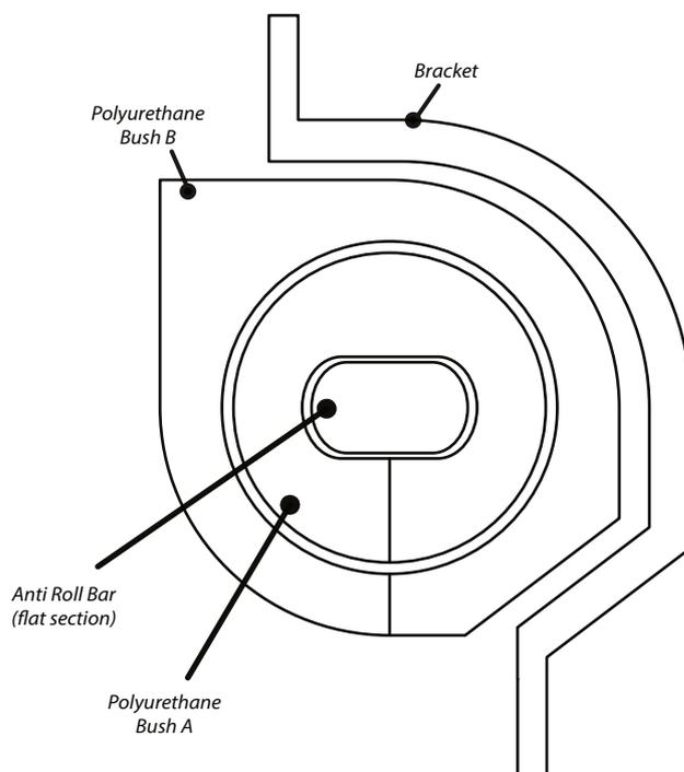
Figure 1- Assembly side profile
